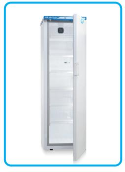
The Labcold ATEX freezer range has been designed with an interior which is licensed as a Zone hazardous area under 2014/34/EU (ATEX Directive) in order to store products which are classed in explosion group IIB+H2 and temperature class T6 under 2014/34/EU (ATEX Directive).
